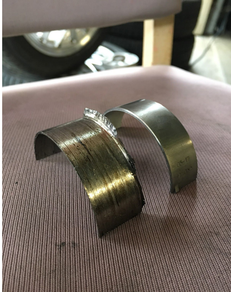
(left: old destroyed bearing, right: new bearing)
