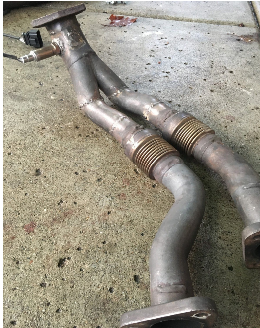
(modified exhaust downpipe)
