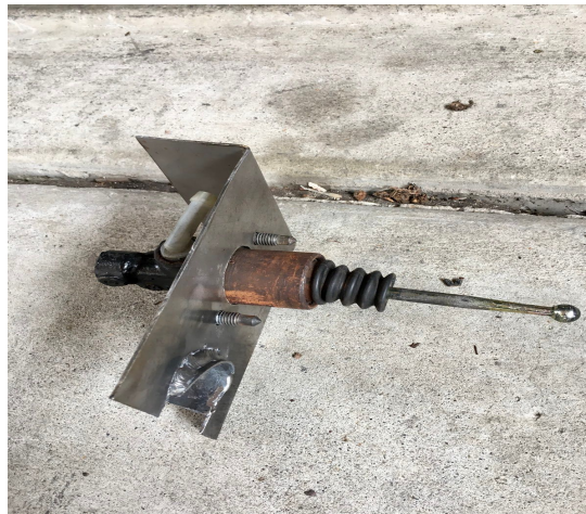
(custom clutch master cylinder bracket)
