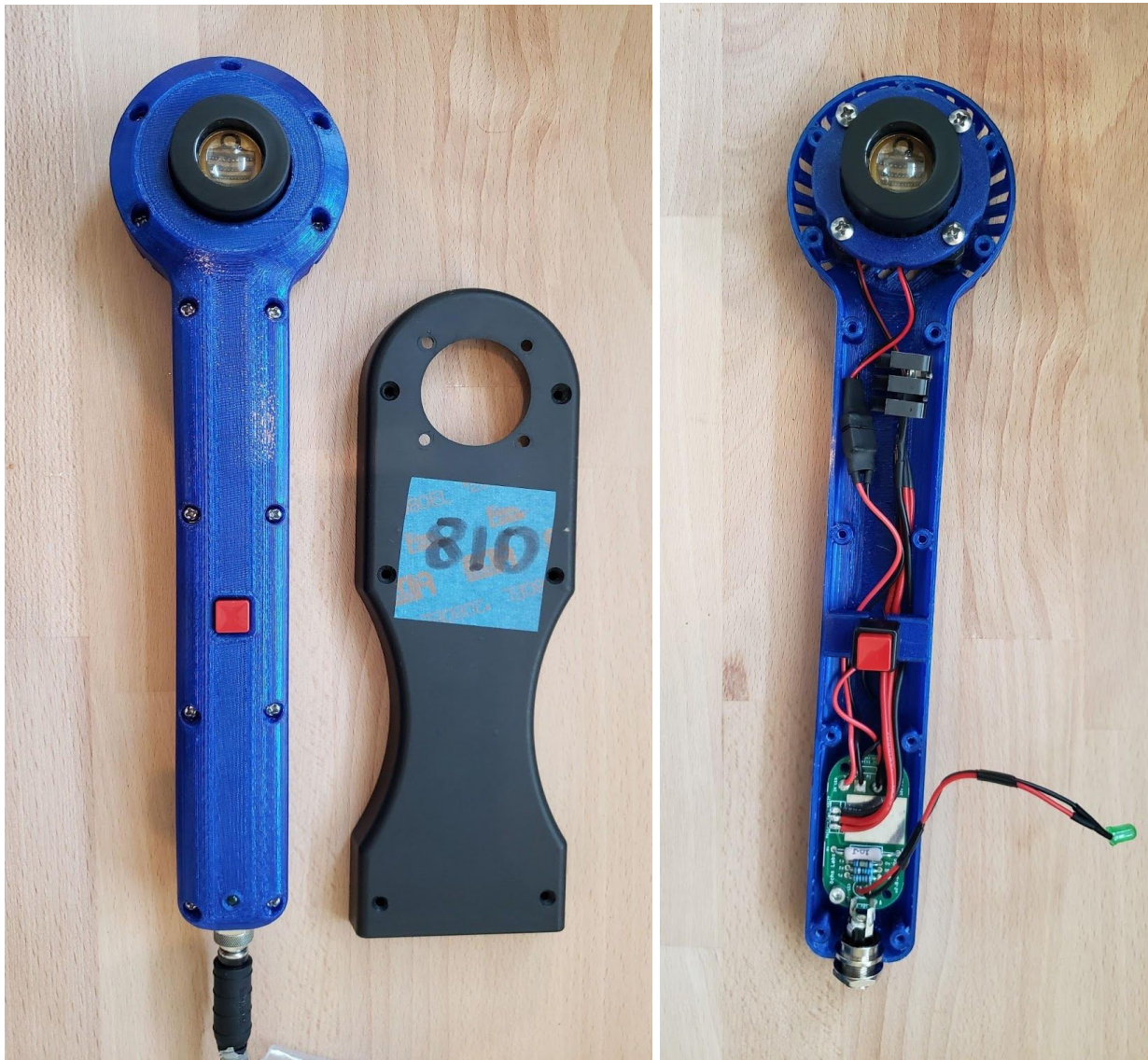
(Left: First fully functional prototype next to original case. Right: Prototype with case removed to showcase internal components.)
