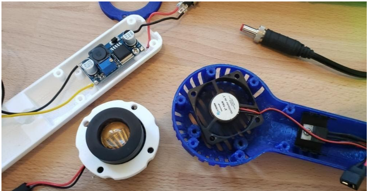
(First and second prototypes open buck converter shown in handle of white case)
