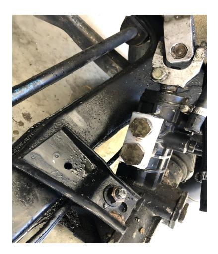
disconnected. Fortunately the power steering system is completely closed so when I removed it it was simply gone, there isn't a lot of blocking off you need to do, the only thing not having it causes you to need on the engine is a different sized belt. After doing this I removed the two banjo bolts from my power steering rack and the tubes attached to them. A few days later my part came, and after fully turning the wheel to each
