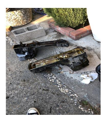
that the sump has a long tube in order to reach all the way back to the deeper section where most of the oil is, while the E34 oil pan doesn't need a long tube as the sump sits right over the deeper section. An oil sump is what sucks oil up and through the engine so everything stays smooth and lubricated, it is chain driven by a little chain that comes down from inside the engine that is connected to the timing directly so whenever the is running or moving how fast
